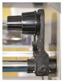
Insert the web into the left support frame, at the first, please confirm the printing side of the web, and then insert the paper tube into the support frame until it can not move. The roll paper tube' diameter include 2.5 inches and 3.5 Inch. You should insert it into the matching support frame (front and rear of the support frame) according to the inner diameter of the paper tube.
