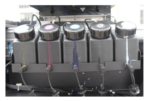
Attention: Please close the valve, when the equipment is not used or replaced for a long time.
