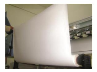
6) Pass material through the platform to reach the front of the machine in a consistent state.
