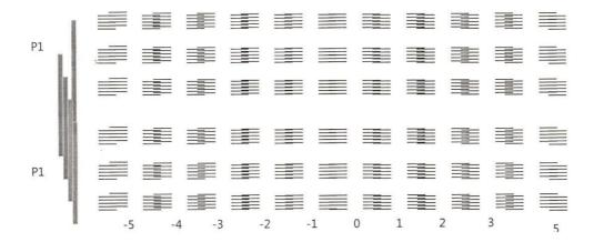
Advanced mode not only provides the media type, but also provides a different PASS number selection. Firstly, adjust the PASS, and its stepping value will correspond to the other PASS. And then adjust 3 PASS, 6 PASS, 8 PASS and other PASS of the same media. And the stepping of other PASS is adjusted on the basis of 4 PASS.
