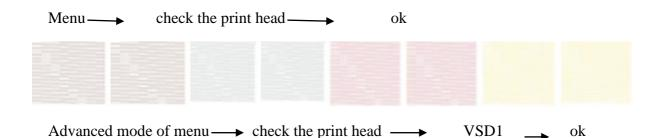
Print 4 different VSD mode test diagram of the print head. Because of the different variable point, the color of the diagram is different.
