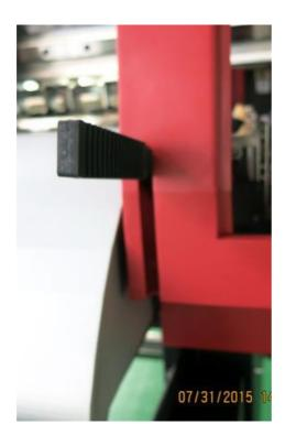
2) Move the support frame on the left (facing the back of the machine) to the far left, tighten the fixing bolts and move the right support frame to the far right (not fixed)
