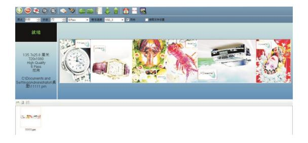
Set the print properties, in the software's real-time parameter settings bar to set the white edge, print speed, print mode (single and double direction) and whether color bars are needed.
