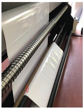
3) Behind the machine, pull out the web 50-60CM
