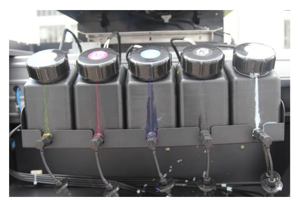
Attention: Please close the valve, when the equipment is not used or replaced for a long time.
